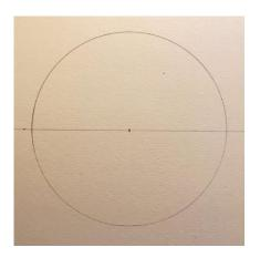
**Step 3** – Keeping the compasses at 6 cm, put the compass point on A and mark arcs above and below on the circumference. Repeat at B.
