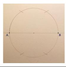
**Step 4** – Using a ruler, join the four arcs and points A and B in turn.
